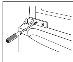
11. Place the upper door back on. Ensure the door is aligned horizontally and vertically so that the seal are closed on all sides before finally tightening the top hinge. Then inert the top hinge and screw it to the top of unit and then fix hinge cover (in accessory bag) by screw.
