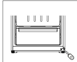
8. Unscrew and remove bottom hinge pin, turn bracket over, and replace it.
