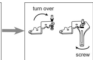
9. Refit the bracket fitting the bottom hinge pin. Replace both adjustable feet. Transfer the lower door to the property position.
