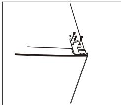
2. Remove the pin with a screwdriver and flip the hinge bracket. Then refit the pin to hinge bracket.
