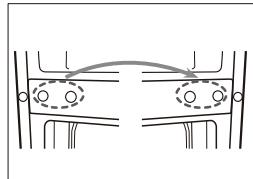
7. Unscrew bottom hinge. Then remove the adjustable feet from both side.
